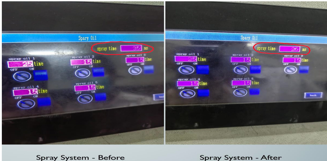
Figure 2 – Pierce Lube Spray Reduction
