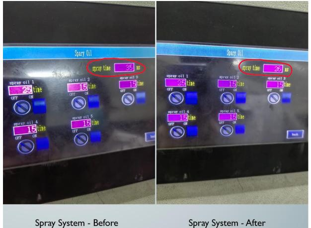
The above picture is an example during testing that we were able to reduce the amount of lubricant spraying into the die at the pierce station. A 9ms reduction in spray time. There was an attempt to reduce the spray even lower, however no spray would come due to low flow rate due to the pressure. At the 26ms spray time, the fins were coming out with the same quality and even less residue than from the competitor's product.
